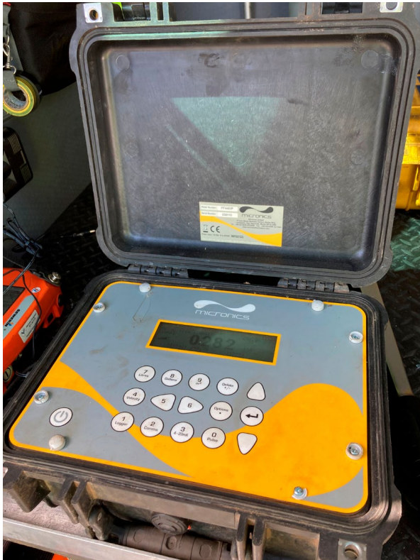
Figur 75. Mottaker for clamp-on-måler (Foto: Marie Sagen)
